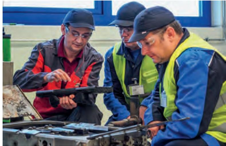
steps can be simulated. The participants can practise all the work stages at the hot end – this is the phase where the glass is moulded.
